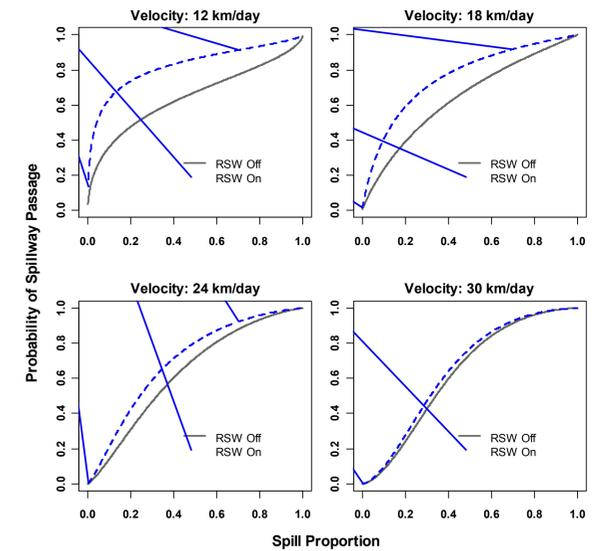
Fig. 4. Predicted SPE functions for steelhead at Lower Granite Dam for RSW on or off under various levels of water velocity.
